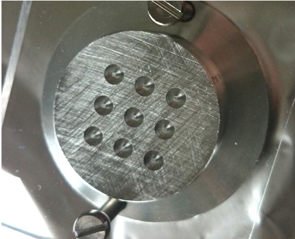
Khatyrka particle sample holder for noble gas analyses
