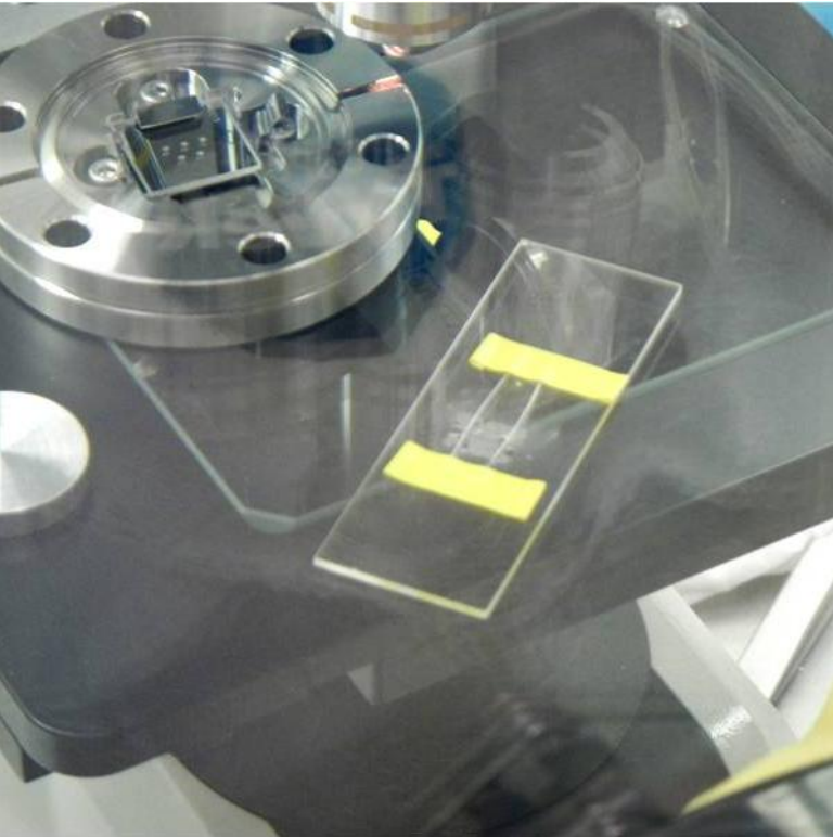
Fishing line's set up for grain transfer from JAXA sample container
