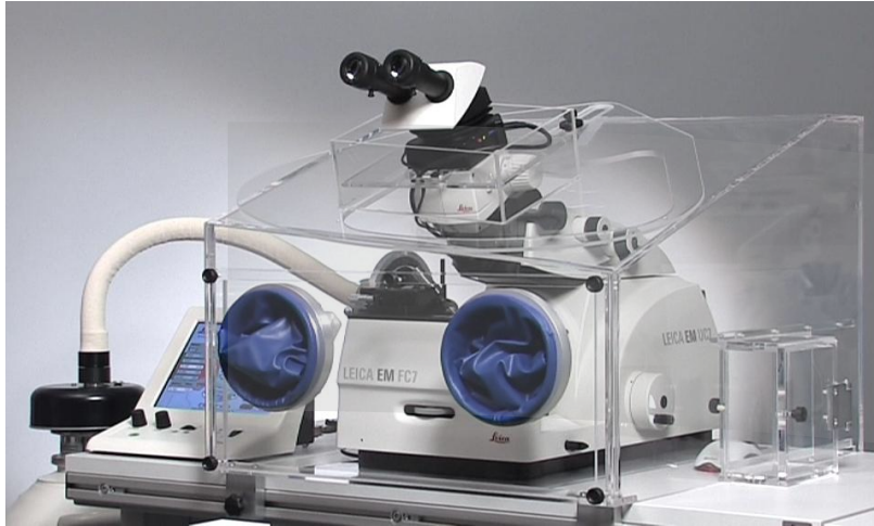
EM FC7 with VCT docking port & "Cryosphere"
