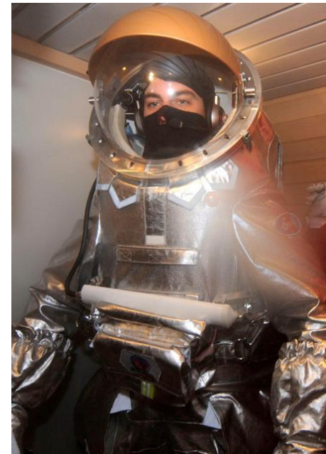
Cryo-chamber test @ -110°C
