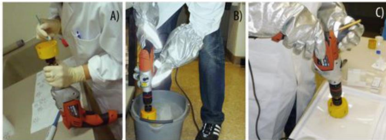
Figure 5: A) Application of the 5.4 \cdot 10^7 microspheres solution. B) Sampling ice core wearing exoskeleton and gloves above. c) Retrieving sample and preparation for further steps.
