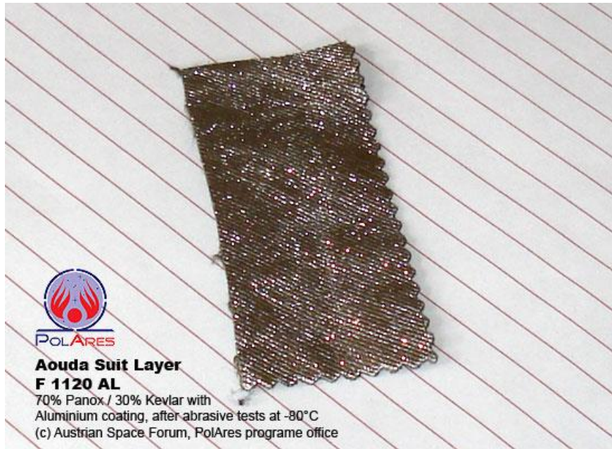
Tissue sample of Inventex® after abrasive tests at -80°C.
