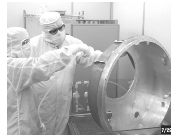
Fig. 4-9. Canister base is rinsed with ultrapure water (UPW)
