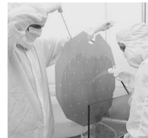
Fig. 4-9. Canister base is rinsed with ultrapure water (UPW)
