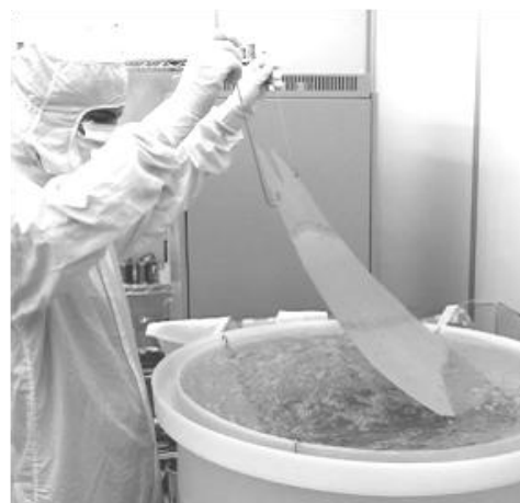
Fig. 4-10. A stream of megasonically energized UPW generated by a portable wand is used to clean the canister base.
